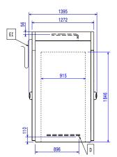
Drain Electrical inlet (power) RO Refrigerant Outlet
